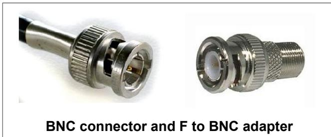
BNC connectors are used on coax cables (sometimes in place of F-connectors). They are commonly found on professional video equipment. Instead of a thread, they use a turn and lock device. As a result they are quicker to connect, provide a cleaner connection, and are less likely to come loose than the push-on RCA-style connectors (see below).
