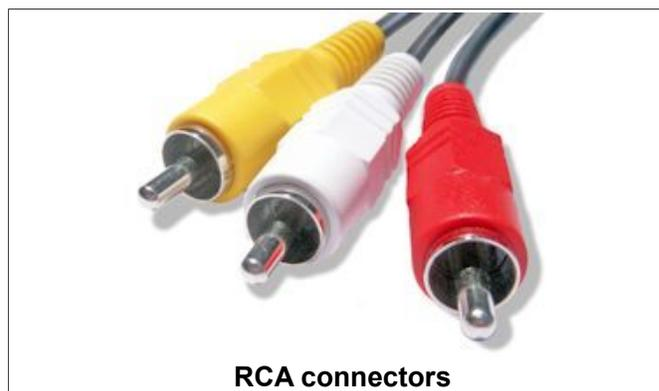
The RCA style connectors are used for both composite analog video and audio. In the old days, these could be found in many colors. In recent times there has been an effort to use yellow for the video signal and red and white for left and right audio. Any color RCA connector will work. The colors simply help keep track of what goes where.
