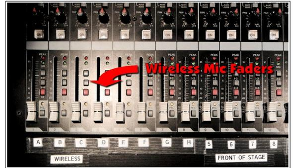
The GTD Audio G-787HL UHF system (A through D) includes two hand held mics and two body packs that can be used with either a head set or lavalier mic.
