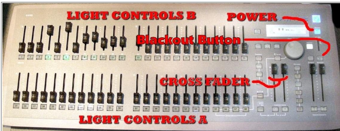
The Smartfade control board has 2 sections of 24 sliders (but only 16 are currently in use) each labeled A and B. The light control board can be set to operate in a fashion similar to the camera mixer. The camera
