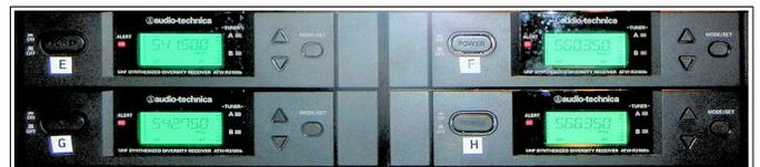
Before using a wireless microphone, check the battery charge indicator (horizontal dashes) in the receiver display. If the battery shows 1 or 2 bars, replace the batteries before using the microphone.
