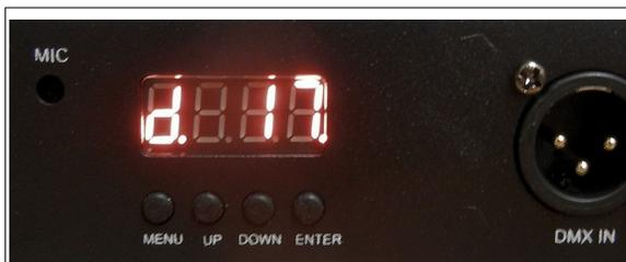
Figure 8: Setting address for Fixture 2.
